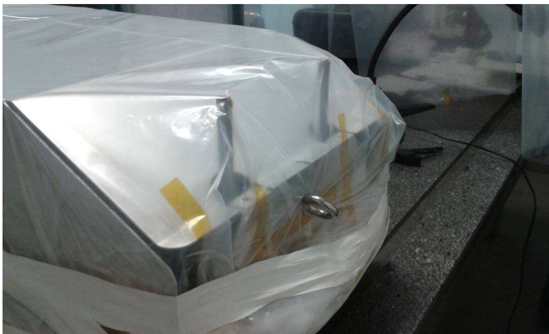
U9 Unscrew the lifting rings
